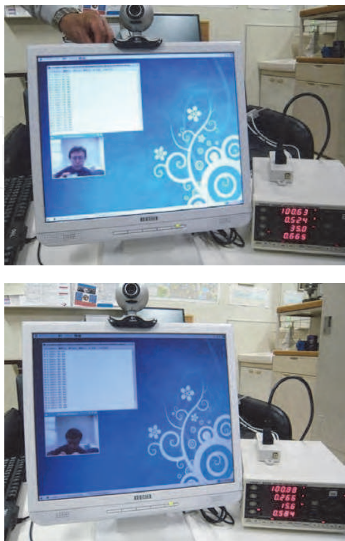
Fig. 10. Screenshots of display and corresponding power consumption: when the user looks at screen, the screen is bright (power: 35W); else the screen is dimmed (power: 15.6W)
