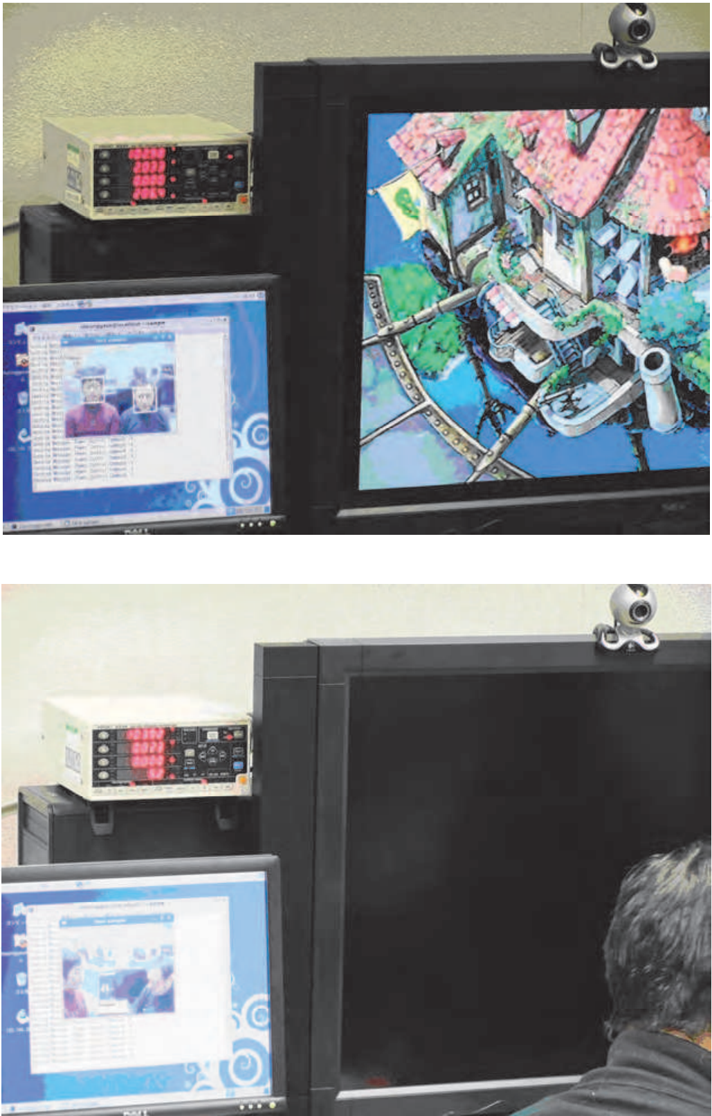
Fig. 15. Screenshots of TV and corresponding power consumption: when viewers looks at screen, the screen is bright (power: 206.4W); else the screen is dimmed (power: 5.2W)
