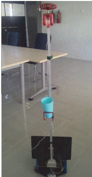
Fig. 11. Prototype of Service robot Srikandi III using stereo camera
