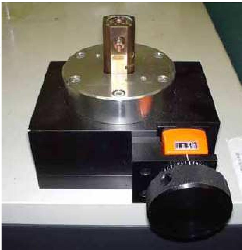
Fig. 3. Schematic picture of diamond anvil cell (DAC).
