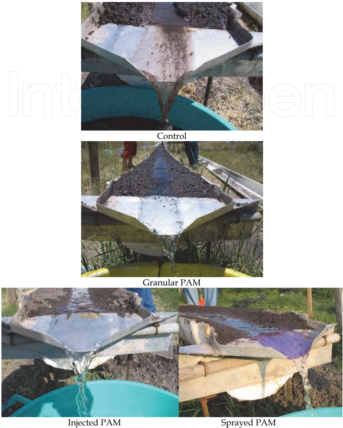
Fig. 5. Detachment in the furrows treatments with PAM and the control
