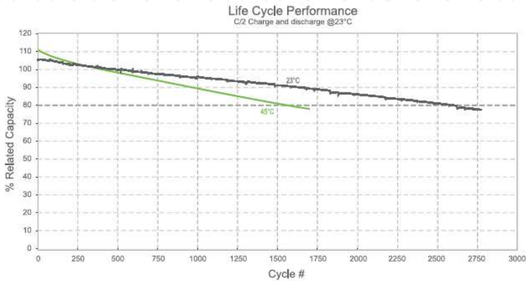
Fig. 6. Battery cycle life depends on operating temperature ( \text{LiFeMgPO}_4 ) (Valence Technology, 2010)
