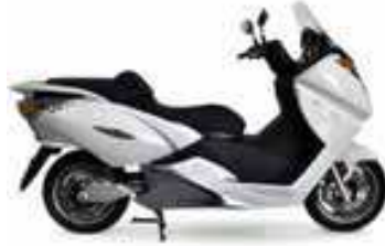
Fig. 14. Battery scooter (Vectrix Corp, 2010) Battery: Li: \text{LiFePO}_4 , 30Ah capacity
