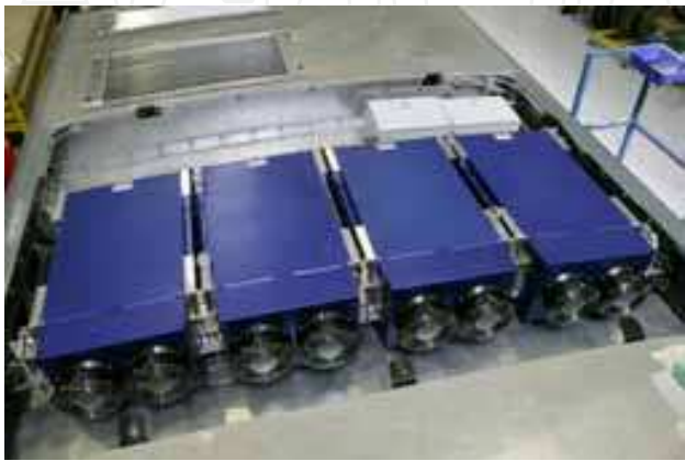
Fig. 21. SC on the roof of Scania bus (Green Car Congress - BioAge Group, 2010)
