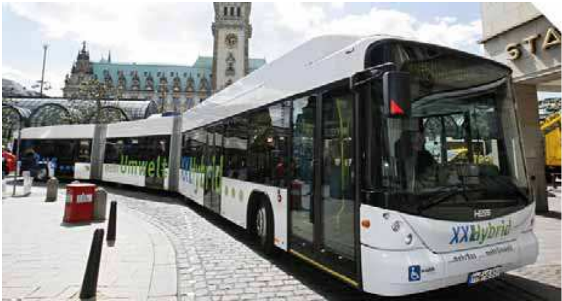
Fig. 19. The hybrid bus with supercapacitors (Maxwell Technologies, 2011)
