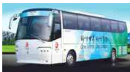
Fig. 16. Battery bus (Zhongtong Bus Holding Co, (n.d.) Battery: Li-ion, 540 Ah capacity
