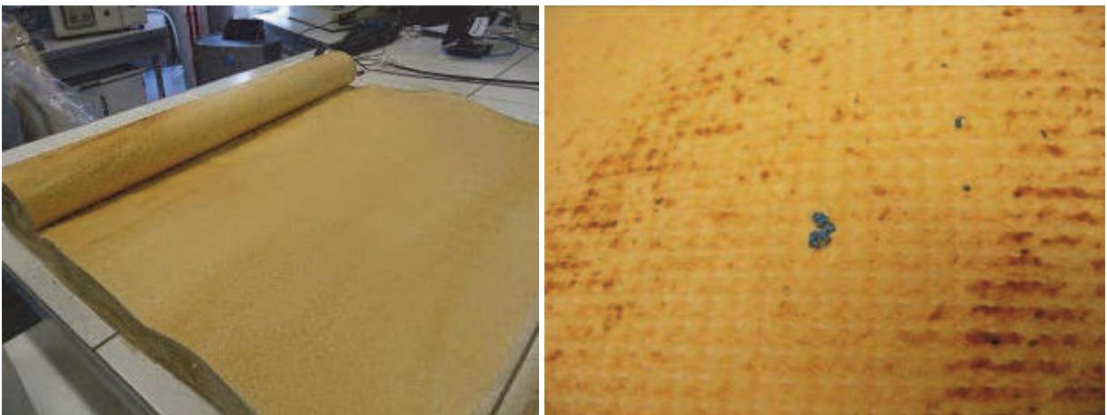
Fig. 8. Iron deposit on RO membrane
