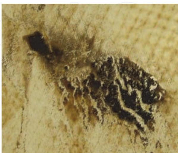
Fig. 10. Deposit of  $\text{MnO}_2$  on RO membrane
