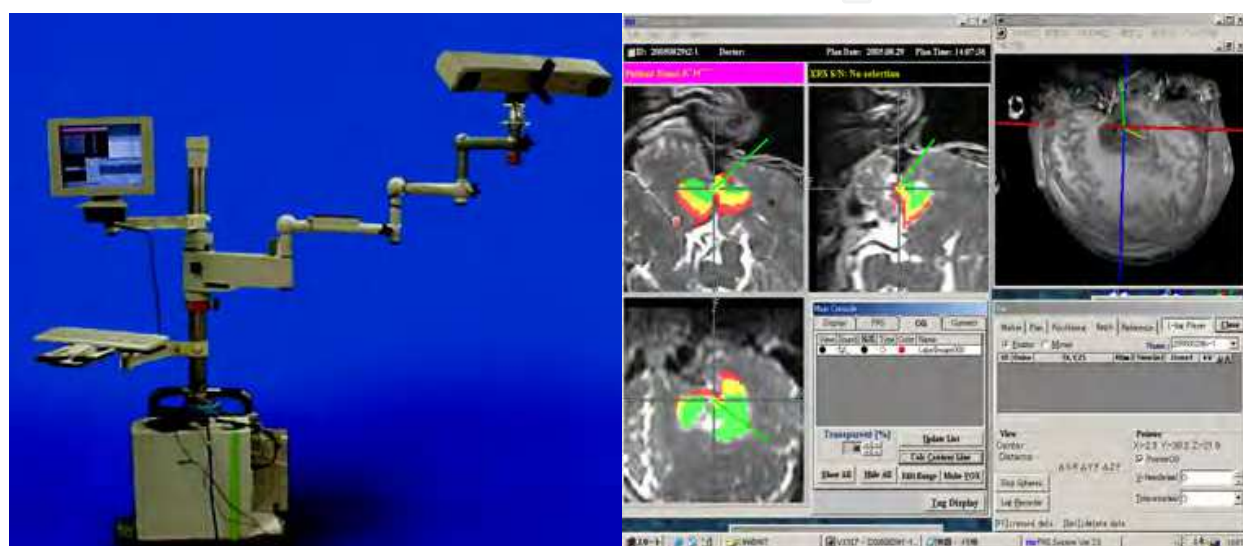
Fig. 5. Intraoperative neuronavigation system (PRS navigator; Toshiba Medical Co. Ltd., Tokyo, Japan) used in intelligent operating theater of TWMU ( left ) and its screen with color-coded safety areas of the tumor resection ( right ), showing areas located less than 5 mm, between 5 and 10 mm, and more than 10 mm to the pyramidal tract, which are demarcated, respectively, as red, yellow, and green.
