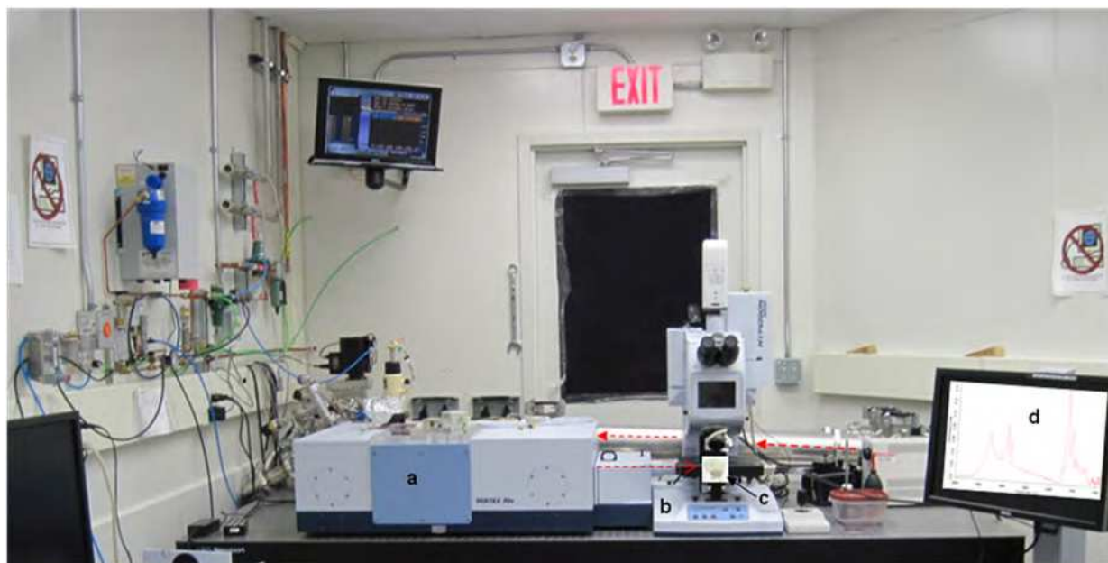
Fig. 5. Experimental hutch, 01B1-1 Mid-Infrared Spectromicroscopy beamline, Canadian Light Source, Saskatoon, Canada. Dotted arrows indicate pathway of synchrotron mid-IR beam entering spectrometer, passing through the tumour specimen, and generating the spectra. a. FTIR Spectrometer, b. spectromicroscope, c. unstained thin tumor section, d. spectra displayed on screen (author's files).
