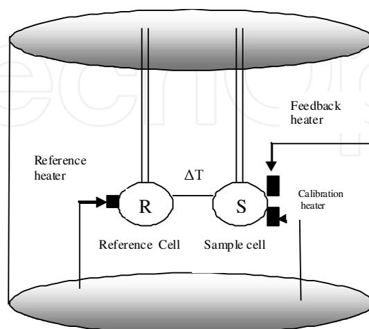
Fig. 1. Schematic diagram of an ITC instrument.
