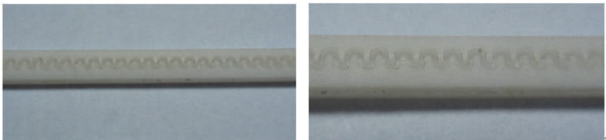
Fig. 37. Oblique teeth channel sheet-dropper products in polyurethane
