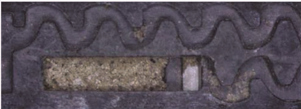
Fig. 29. Clogging status in the optimized emitter
