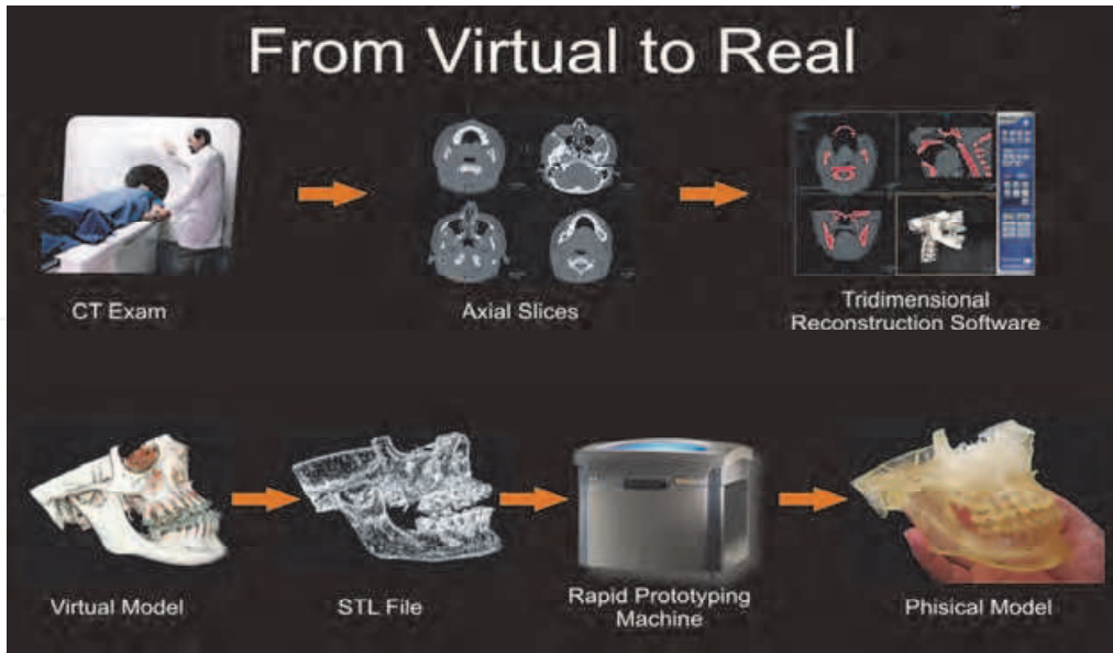
Fig. 12. Step by step sequence to fabricate a prototype of a human anatomic structure * Attention: to fabricate the prototype, images should be stored in DICOM format and recorded in a CD-ROM or sent via the Internet to the prototyping bureau; the CT scan films are not necessary.
