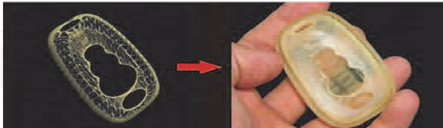
Fig. 1. Virtual file and corresponding prototype built using rapid prototyping.
