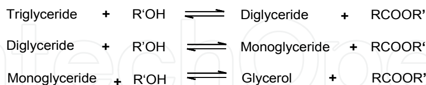
Fig. 2. Chemistry of transesterification process
