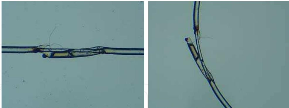
Fig. 15. Image of the fiber bend section, after being submitted to an optical power of 1.5W. The bending diameter was 2.9mm and the exposure time was 60 s (magnification of X5)
