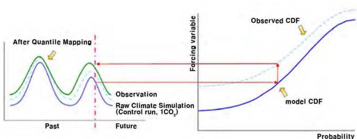
Fig. 3. Quantile mapping.
