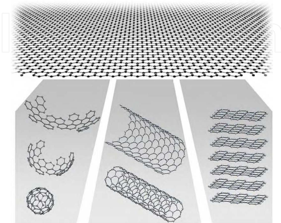
Fig. 2. **Mother of all graphitic forms.** Graphene is a 2D building material for carbon materials of all other dimensionalities. It can be wrapped up into 0D buckyballs, rolled into 1D nanotubes or stacked into 3D graphite [from: Geim and Novoselov, <http://arxiv.org/ftp/cond-mat/papers/0702/0702595.pdf>]
