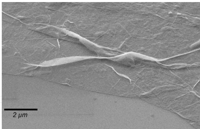
Fig. 3. A few layers of graphene seen by scanning electron microscopy [Taken from [www.sineurop-nanotech.com/en/graphene.html](http://www.sineurop-nanotech.com/en/graphene.html) Courtesy SINEUROP Nanotech GmbH, Stuttgart, Germany]
