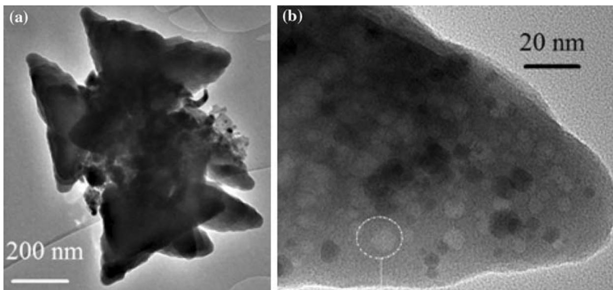
Fig. 13. (a) Low magnification TEM of the triangular envelopes of  $\text{VO}_x$ , (b) one pocket at higher magnification, showing the small voids and solid spheres. The spheres have been found to be inorganic fullerenes of  $\text{VO}_x$  segregated from graphene sheet that forms the envelope [52].
