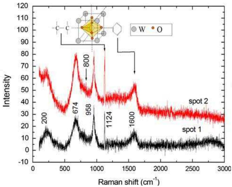
Fig. 14. Raman spectra of metal oxide QD-functionalised graphene. The G peak at  $1600\text{ cm}^{-1}$  and the  $G'$  at  $2700\text{ cm}^{-1}$  on spot 1 are signatures from graphene layers. The rest of the peaks are from the metal oxides ( $\text{VO}_2$  and  $\text{WO}_3$ ) [52]
