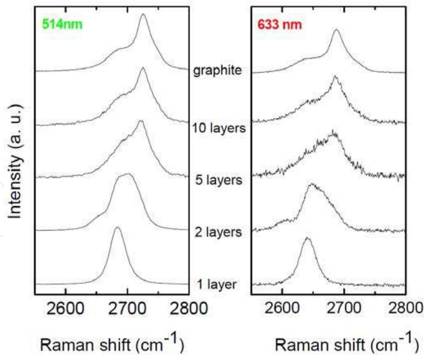
Fig. 6. Raman spectra under 514 nm and 633 nm laser wavelength excitation of the G' for different number of layers showing the single  $2690\text{ cm}^{-1}$  phonon from the one-layer graphene replaced by a main phonon at  $2710\text{ cm}^{-1}$  with the  $2690\text{ cm}^{-1}$  becoming its shoulder in multi-layer graphite (From A.C. Ferrari et al [7])
