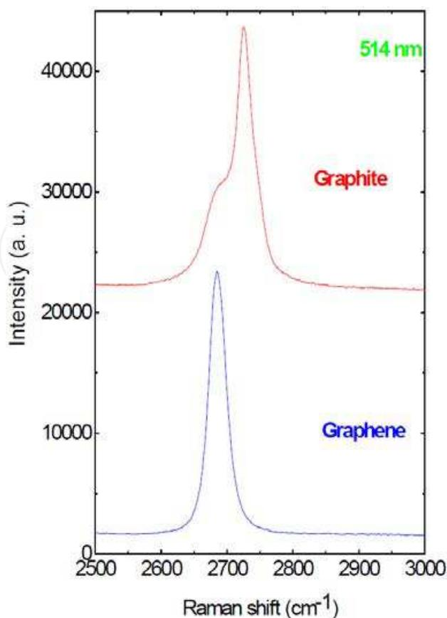
Fig. 7. The single 2690  $\text{cm}^{-1}$  phonon from the one-layer graphene replaced by a main phonon at 2710  $\text{cm}^{-1}$  with the 2690  $\text{cm}^{-1}$  becoming its shoulder in multi-layer graphite (From A.C. Ferrari et al [7])
