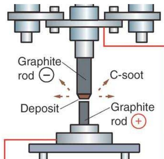
Fig. 11. A typical arc discharge system [mrsec.wisc.edu/.../images/nanotubes/arc.jpg]
