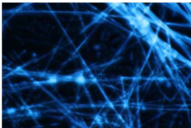
Fig. 5. Optical image of fluorescent self-assembled peptide nanostructures. The nanotubes were functionalized with salicylic acid in order to enhance its fluorescence following the method developed by (Ryu et al., 2009).
