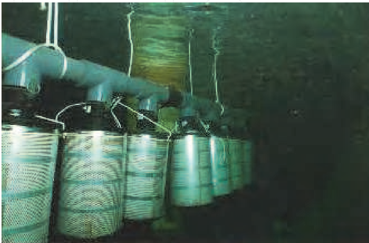
Fig. 4. UCC vacuuming filtration system underwater manifold.
