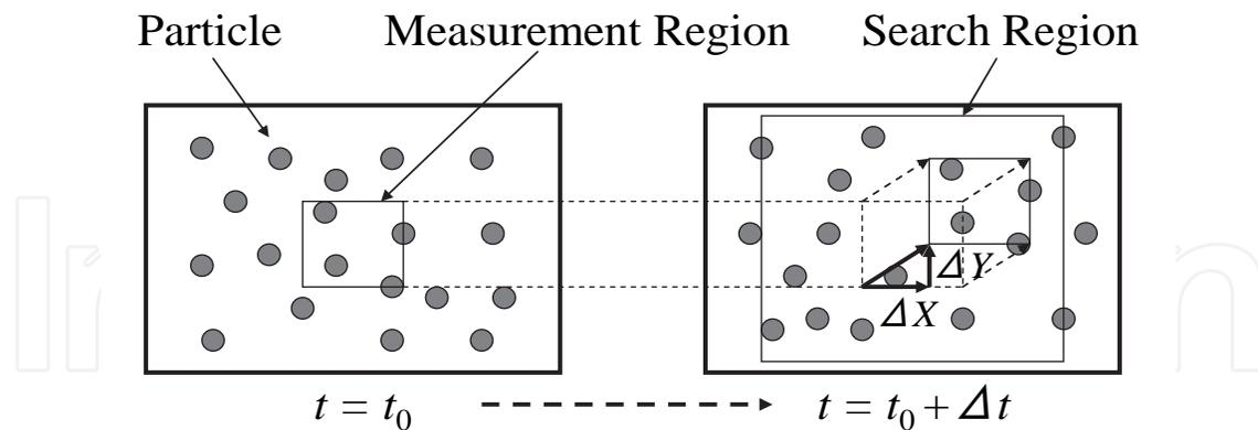
Fig. 3. Principle of determining velocity through PIV.
