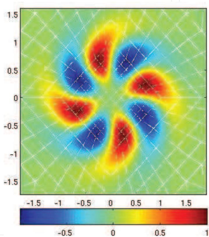
Fig. 8. Axial component of the disturbance velocity of one of the unstable modes (four lobes) of a isolated Batchelor vortex at  $Re = 667$  and  $\beta = 2.0$ .
