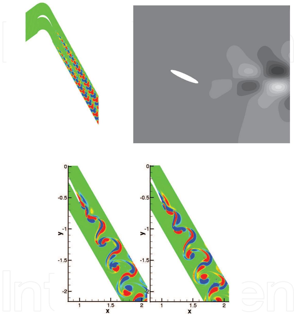
Fig. 11. *Upper-Left*: Leading eigenmode in the wake of the T106-300 LPT flow at  $Re = 890$ . *Upper-Right*: Leading (wake) eigenmode in flow over an aspect ratio 8 ellipse at  $Re = 200$  Kitsios et al. (2008). *Lower*: Leading LPT Floquet mode at  $Re = 2000$  Abdessemed et al. (2004).
