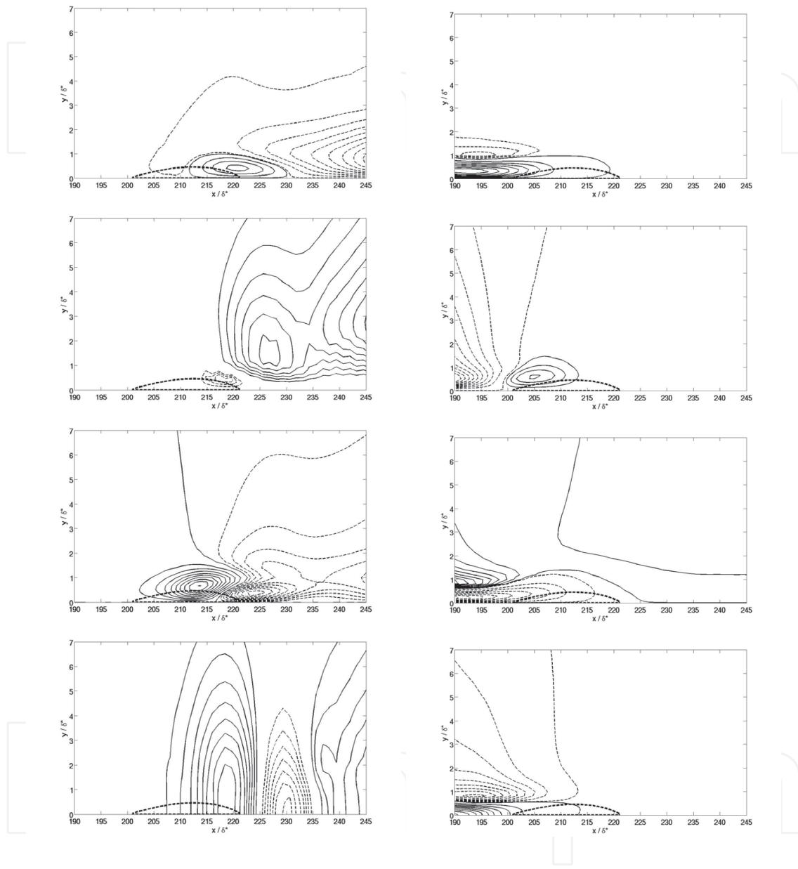
Fig. 2. Most unstable steady global mode for the direct and adjoint problem at  $Re_{\delta^*} = 500$  and  $\beta = 0.2$ . The real streamwise (*first row*), wall-normal (*second row*) and spanwise (*third row*) velocities and pressure (*forth row*) components of the direct (*left column*) and of the adjoint (*right column*) eigenfunctions are shown. The thick dashed line separates the reversed flow region. Only a part of the domain is shown.
