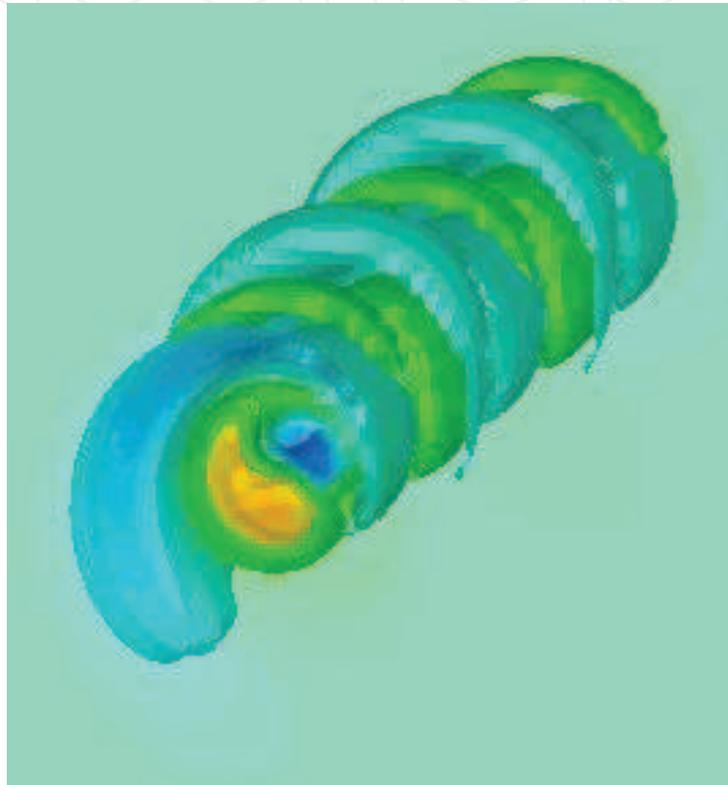
Fig. 7. Superposition upon the steady laminar basic state at  $Re = 3180$ ,  $U_0 = \frac{0.5}{\pi}$ , of its most amplified BiGlobal eigenmode at amplitude 0.1%. Axial spatial direction reconstructed using  $L_x = 2\pi/\beta$ , with  $\beta = 3.0$ ; eigenvalue  $\omega_i = 0.04603$ ,  $\omega_r = 0.06072$  González, Gómez-Blanco & Theofilis (2008).
