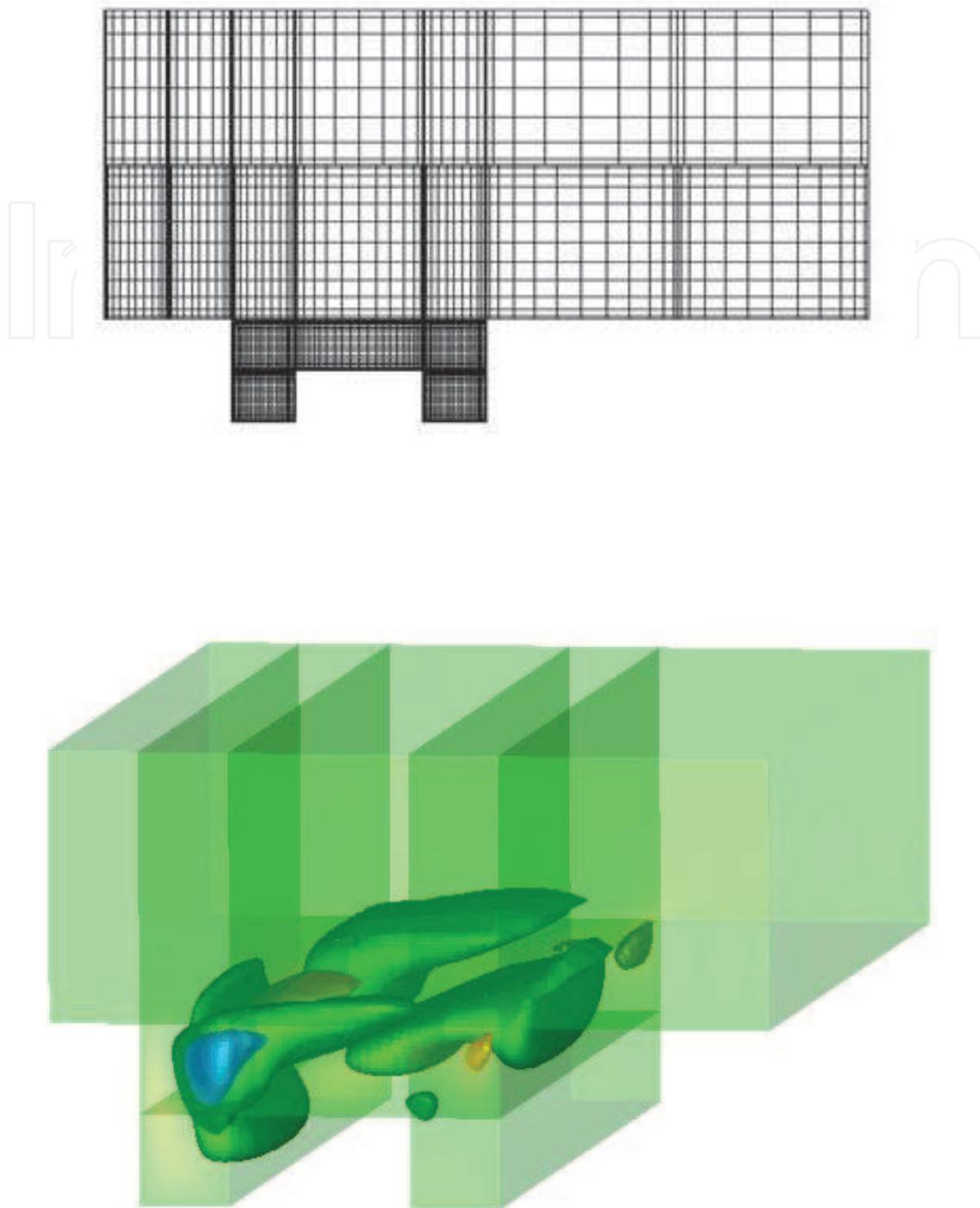
Fig. 6. *Upper*: Non-conforming spectral multidomain discretization of an open-cavity configuration, containing a rectangular object. *Lower*: Perspective view of the least-damped eigenmode of incompressible flow at  $Re = 400$  de Vicente et al. (2006).
