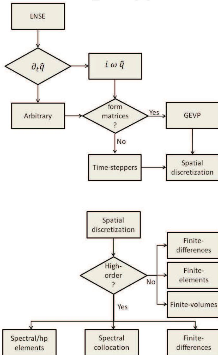
Fig. 1. *Upper:* Treatment of the temporal derivative in a global instability analysis context. *Lower:* Numerical methods which have been used for the spatial discretization of global instability eigenvalue problems.
