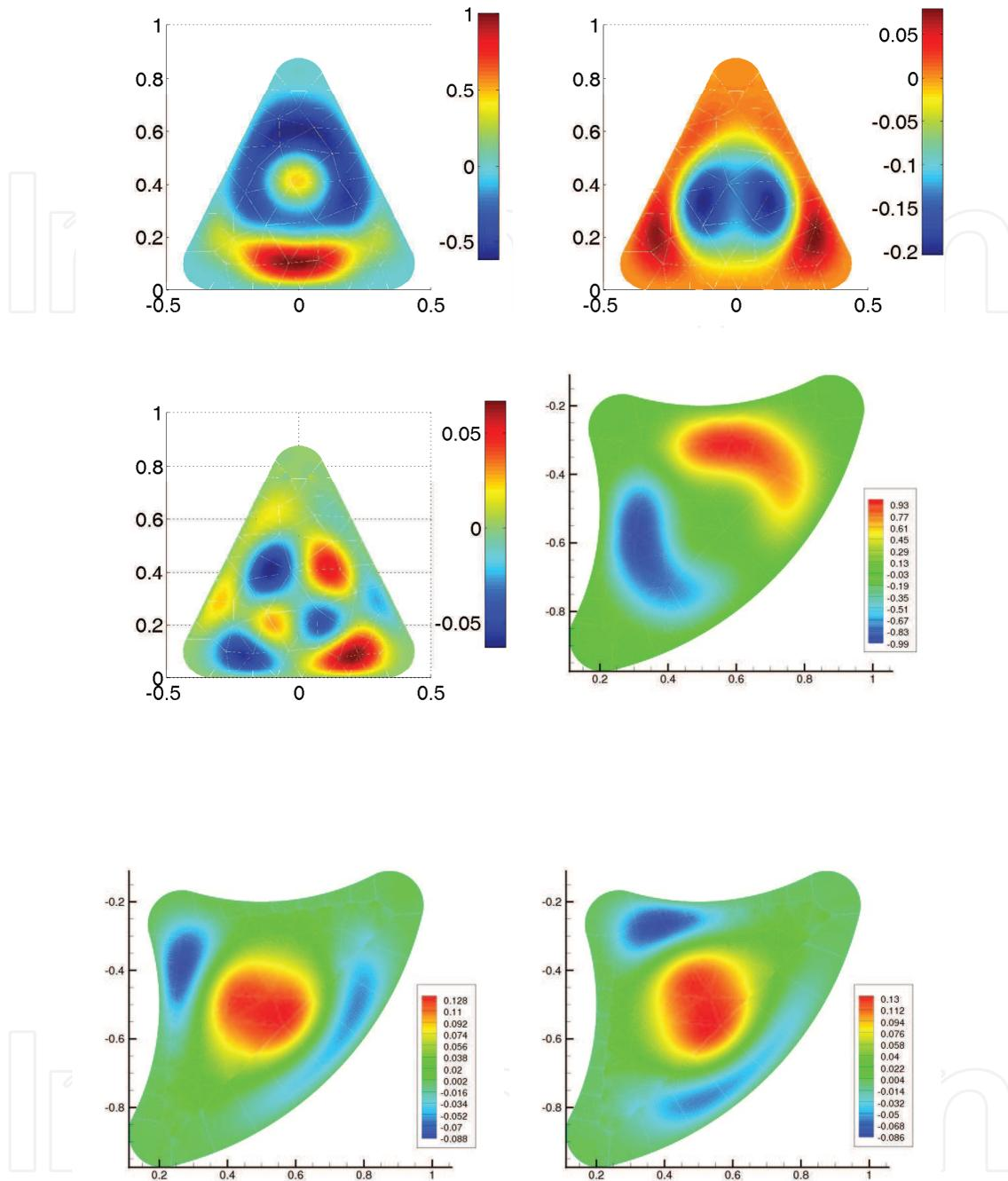
Fig. 10. *Upper*: Amplitude functions of the least-damped eigenmode of geometry "in<sub>1</sub>" at  $Re = 1000$ ,  $\alpha = 1$  González, Rodríguez & Theofilis (2008). *Lower*: Amplitude functions of the least-damped eigenmode of geometry "in<sub>2</sub>" at  $Re = 1000$ ,  $\alpha = 1$  González, Rodríguez & Theofilis (2008). Left to right column:  $\hat{u}_1$ ,  $\hat{u}_2$ ,  $\hat{u}_3$ .
