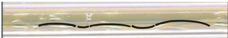
Fig. 10.2a. Liquid behaviour of the butanol aqueous solution (7.15 wt%) (Run 2a).
