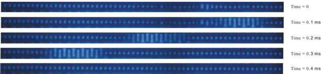
Fig. 10. Elongated slug bubble flow at G = 267 kg/m 2 s, q'' = 565.9 kW/m 2 , and x = 0.14
