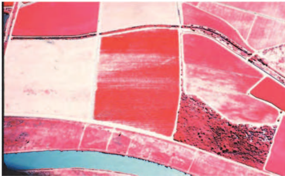
Fig. 12. Example of image processing of aerial infrared photographs to produce a vegetation map for a Chile field.
