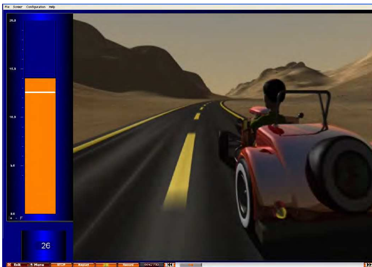
Fig. 6. An example of a computer screen where the mean amplitude of the EEG frequency of interest is fed back to the client via an orange bar graph with a white criterion line. In addition, a film clip and a counter are shown as rewards for the client.
