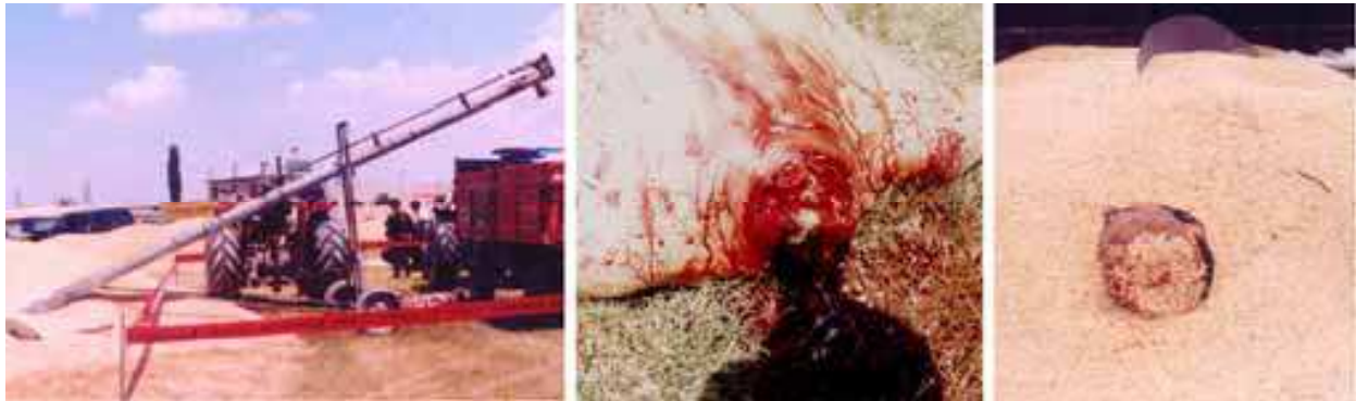
Fig. 26. A 41-year-old male farmer was found decapitated in the stackyard. He was working with a helix elevator machine. He had scarf tied loosely over his face and neck but the scarf was pulled up and wrapped around the shaft of the machine. The scarf then slid around the victim's neck and tightened, causing the head to separate from the body.
