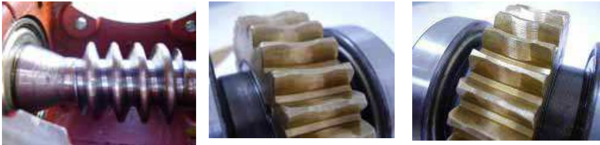
Fig. 15. Inner elements of the reducer after the first test.
