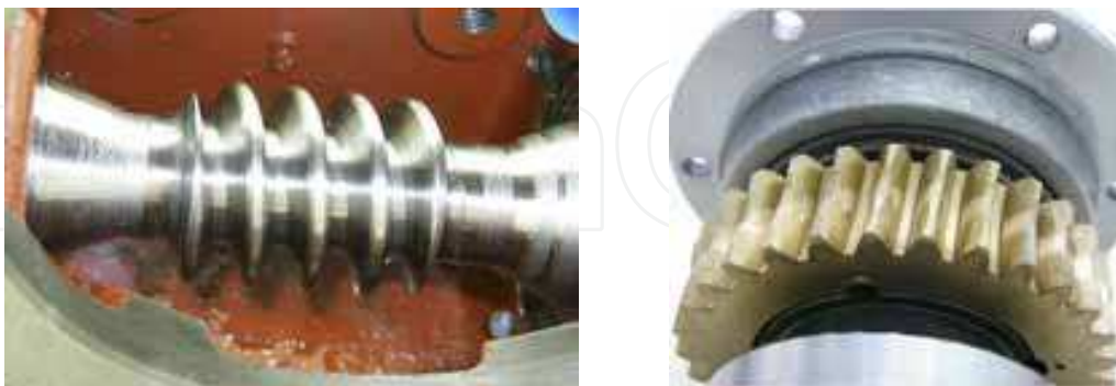
Fig. 10. Inner elements of the reducer. On the left is the worn screw and on the right the crown gear.
