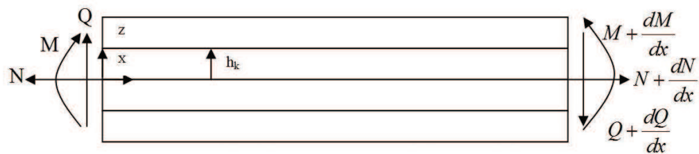
Fig. 1. Free body diagram of a differential beam element
