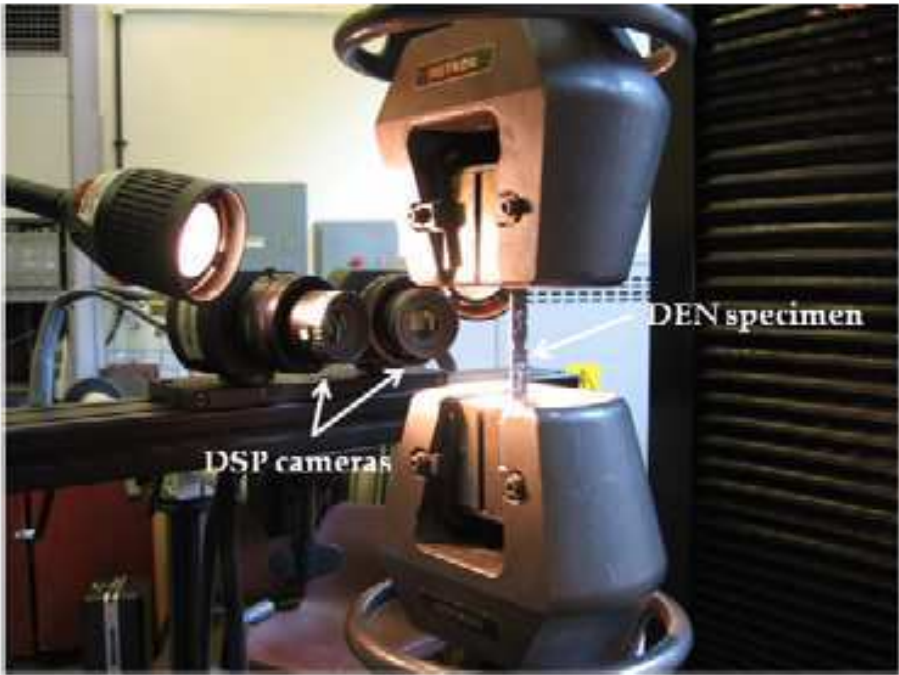
Fig. 9. Experimental setup for DEN specimens
