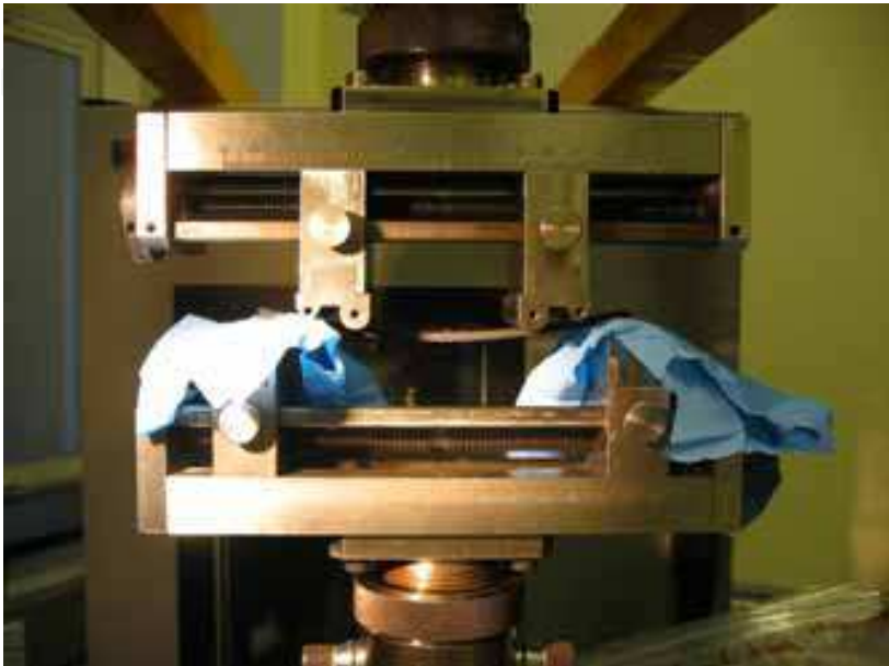
Fig. 10. Experimental setup for 4PBT specimens
