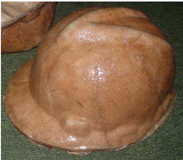
Fig. 11. Preliminary design safety helmet ramie-garut biocomposite
