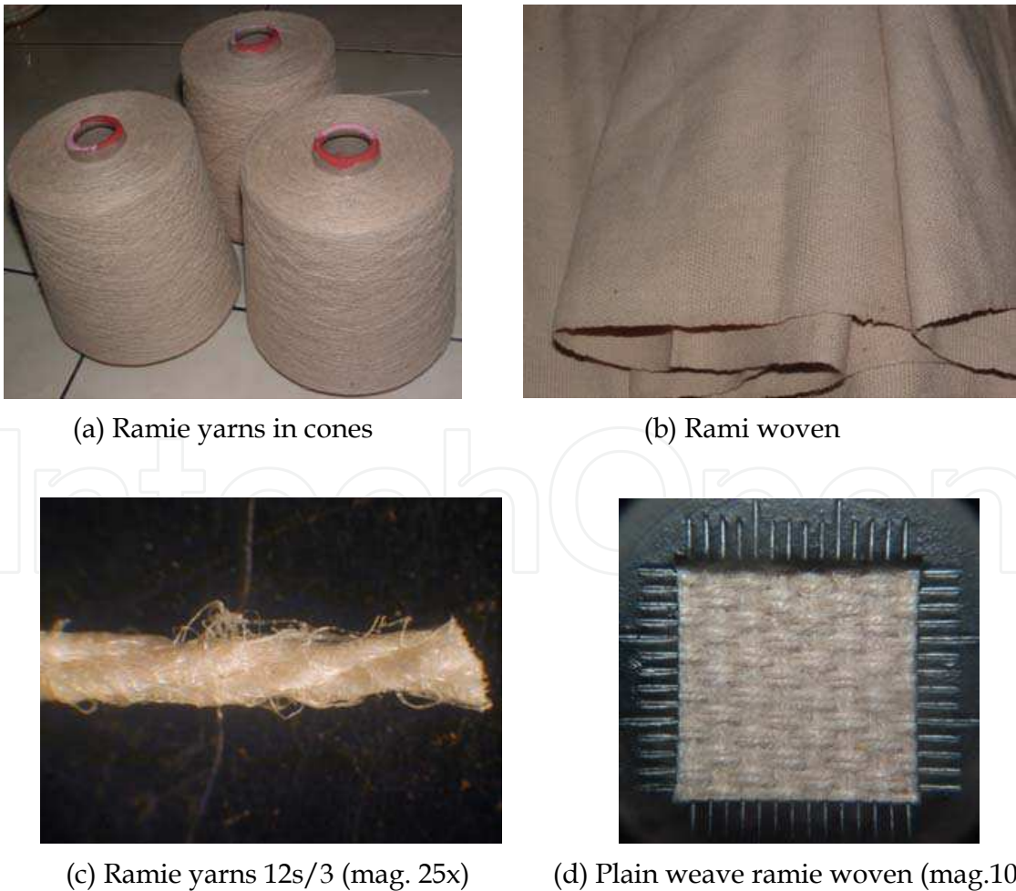
Fig. 2. Ramie woven structure
