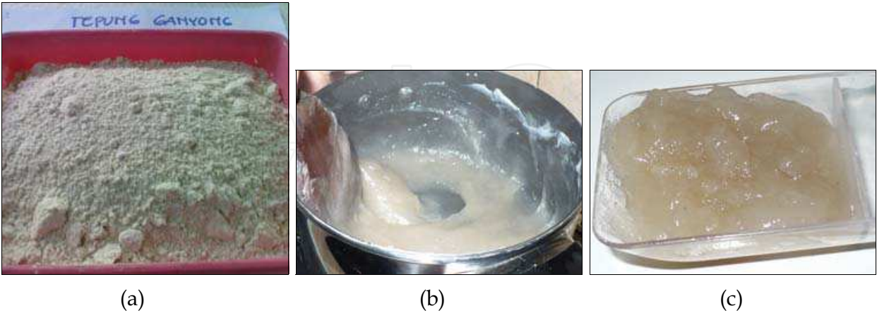
Fig. 4. Making biosizing for matrix in biocomposite system. (a) starch based material for sizing; (b) Gelatinised starch; (c) biosizing ready to use
