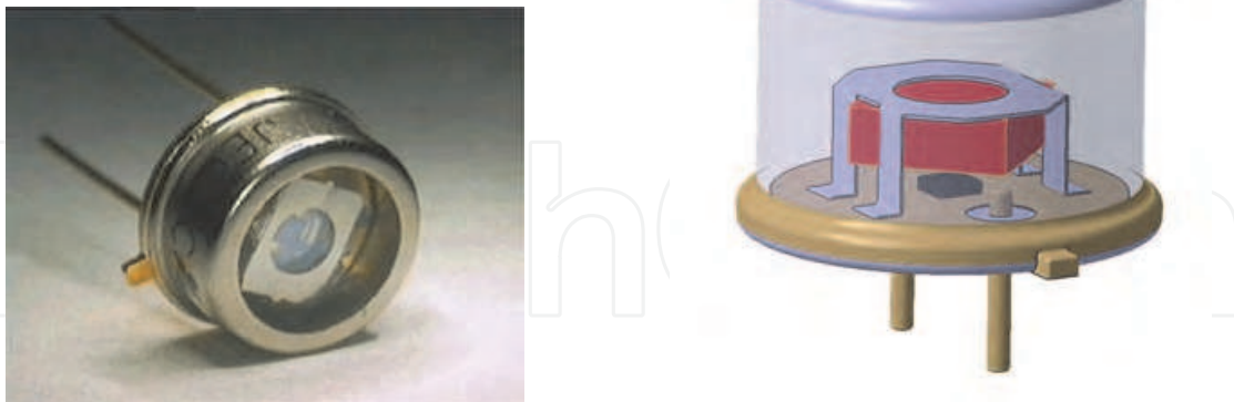
Fig. 1. (Left) Commercial hermetically sealed filtered ultraviolet (UV) photodiode with TO5 housing and the filter mounted on a metallic platform. (Right) Geometrical configuration of the photodiode. The filter crystal is here represented in red and the SiC detector dice in black. The filter is mounted on the metallic structure but does not reach the side of the housing.
