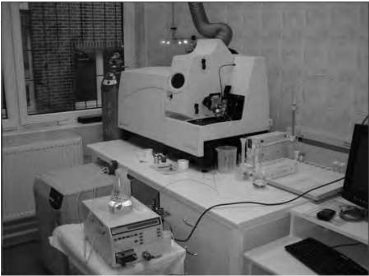
Fig. 2. The applied inductively coupled plasma mass spectrometer
