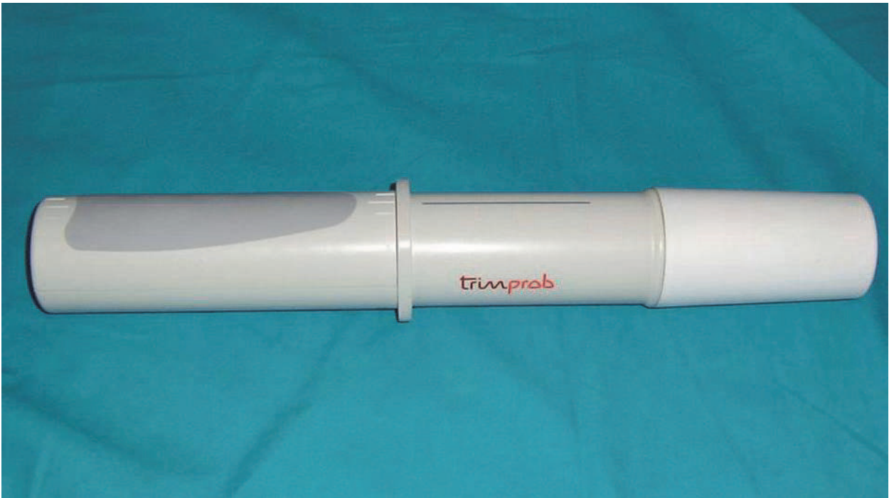
Fig. 2. Hand-held, battery-operated detection probe.
