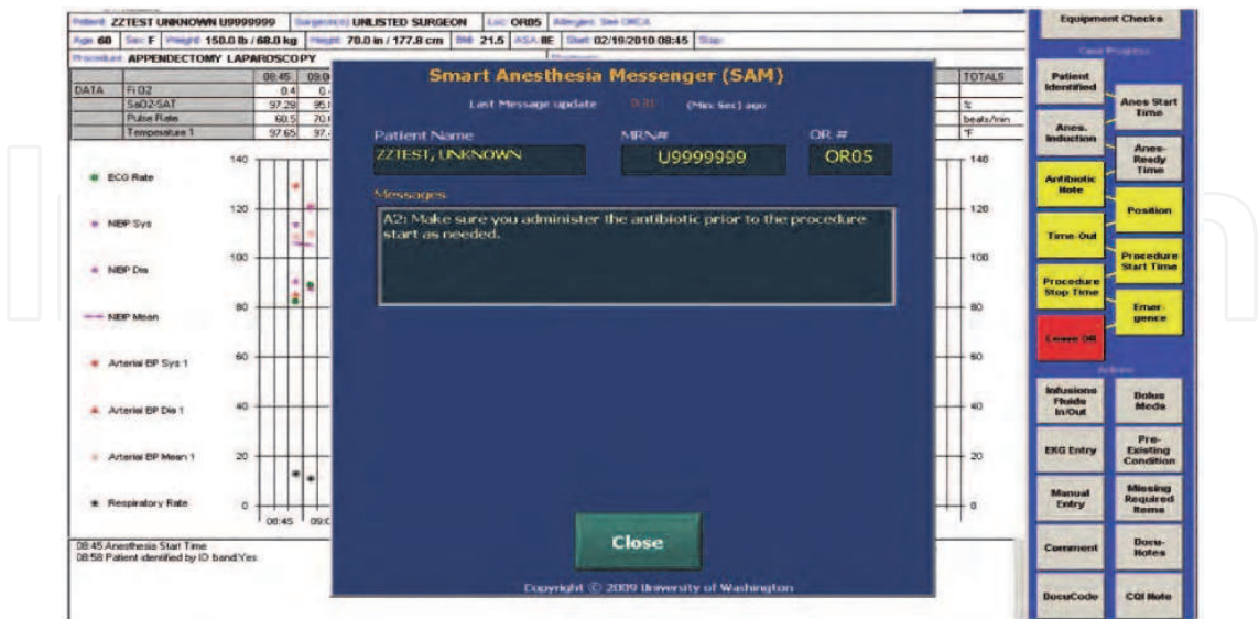
Fig. 12. Smart Anesthesia Messenger (SAM) alert screen overlaid on anesthesia information management system screen. (Nair et al., 2010)
