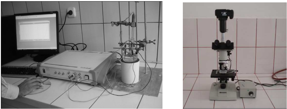
Fig. 40. Electrochemical assembly used for corrosion tests and the metallographic microscope type EUROMEX
