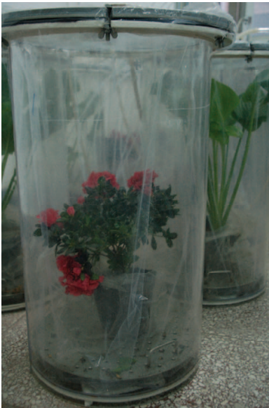
Fig. 3. Photograph of a Plexiglas chamber housing one potted plant
