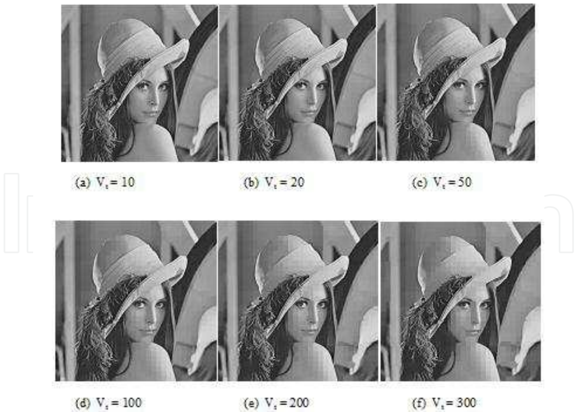
Fig. 1. Reconstructed Lena images with compressed 16*16 blocks with different threshold variances V_t .
