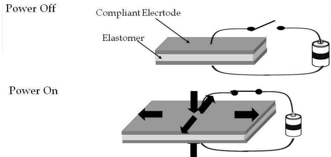
Fig. 3. Principle of operation of dielectric elastomers
