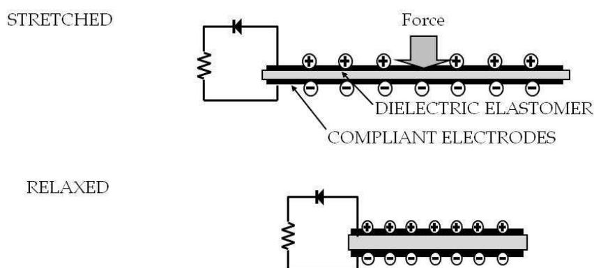
Fig. 7. Operating principle of dielectric elastomer power generation
