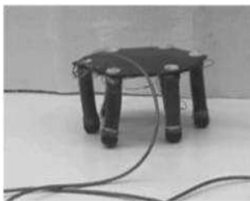
Fig. 4. Biologically inspired robots powered by dielectric elastomer rolls (Pei et al, 2003; Chiba et al, 2006a). (a) Role Actuator Having 3-DOF (b) Application example to a robot: it enables sideways stepping like a crab without turning around, when it collides with wall
