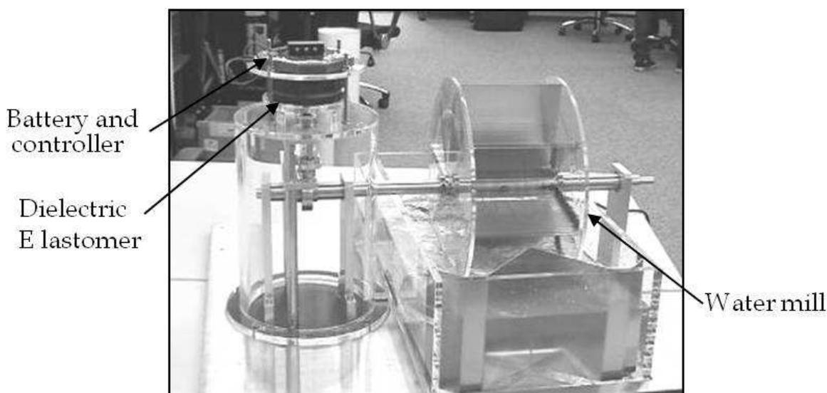
Photo 7. Water mill generator using dielectric elastomer
