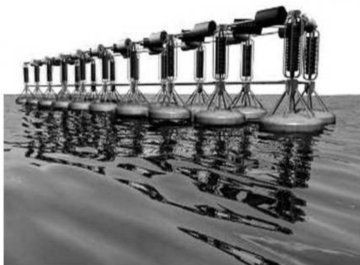
Fig. 14. Conceptual rendering of wave power generator system using dielectric elastomers
