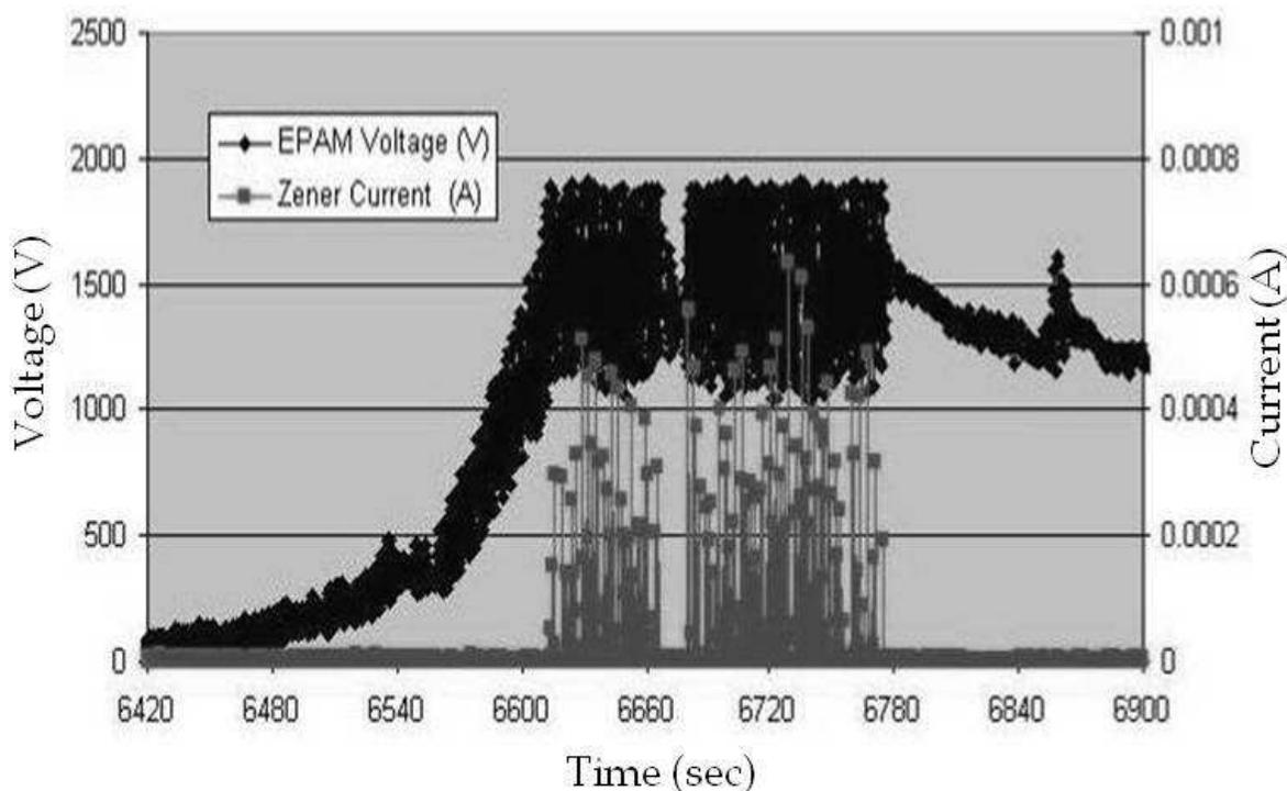
Fig. 11. Electricity generated by ten centimeter-high waves
