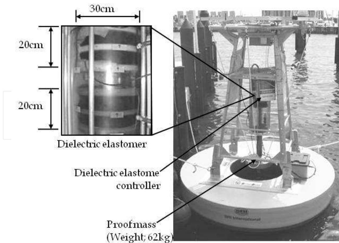
Photo 6. Dielectric elastomer generator on the test buoy
