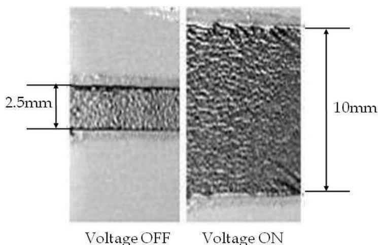
Photo 1. Acrylic elastomers showing 380% linear strain
