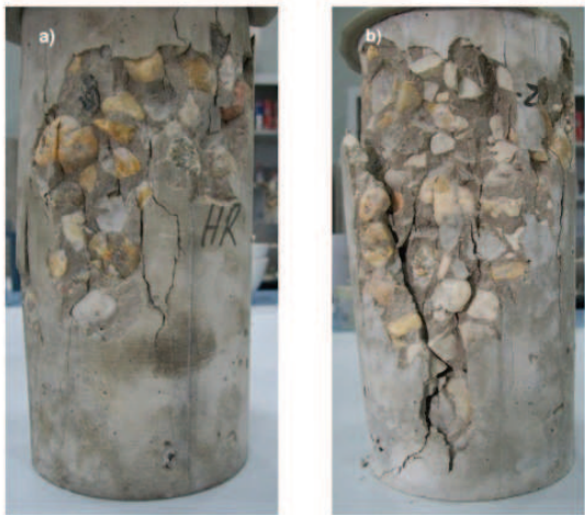
Fig. 3. Types of compressive fracture: a) Concrete CC. b) Recycled concrete RC-25
