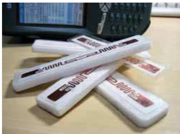
Fig. 2. Displayed the UHF RFID tags using in the case study.
