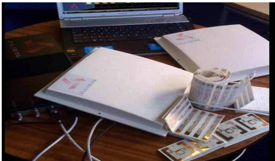
Fig. 4. The Alien RFID Reader, Antenna and Tags
