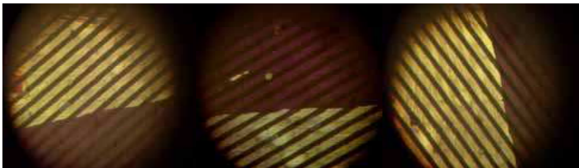
Fig. 6. Images of the DBPI film grown on the \text{NdGaO}_3(001) substrate at different orientations of the films relative to crossed polarizers.
