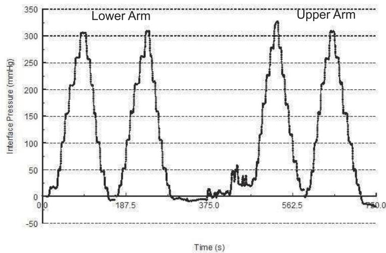
Fig. 6. Interface pressure measured under 10 cm Zimmer Cuff on Lower and Upper Arm
