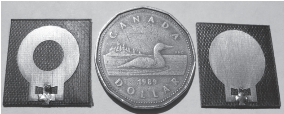
Fig. 18. Circular monopole antennas of Fig. 3a and Fig. 3c etched each on a 22x22mm 2 substrate with \epsilon_r=2.5 , height=0.8mm. Antennas are compared to the Canadian Dollar Coin before being mounted on the Aluminium ground plane
