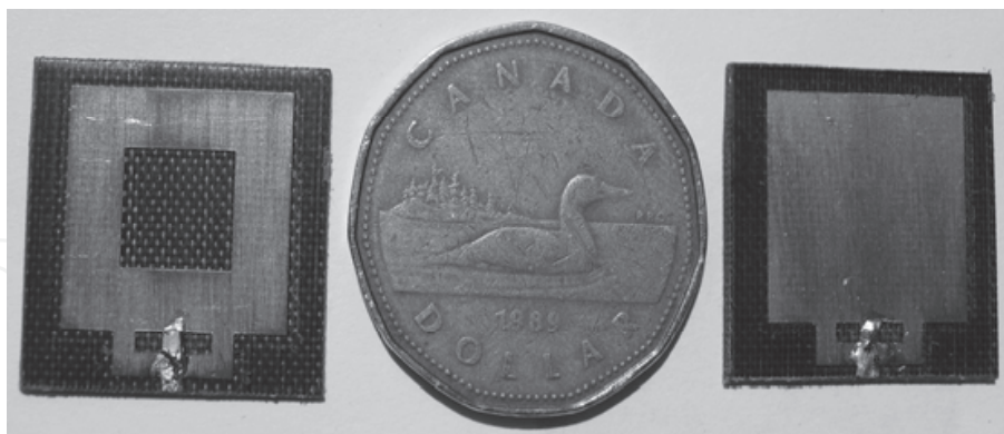
Fig. 16. Square monopole antennas of Fig. 1a and Fig. 1c etched each on a 22x22mm 2 substrate with \epsilon_r=2.5 , height=0.8mm. Antennas are compared to the Canadian Dollar Coin before being mounted on the Aluminium ground plane
