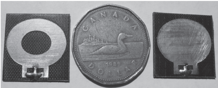
Fig. 20. Elliptical monopole antennas of Fig. 5a and Fig. 5c etched each on a 22x22mm 2 substrate with \epsilon_r=2.5 , height=0.8mm. Antennas are compared to the Canadian Dollar Coin before being mounted on the Aluminium ground plane
