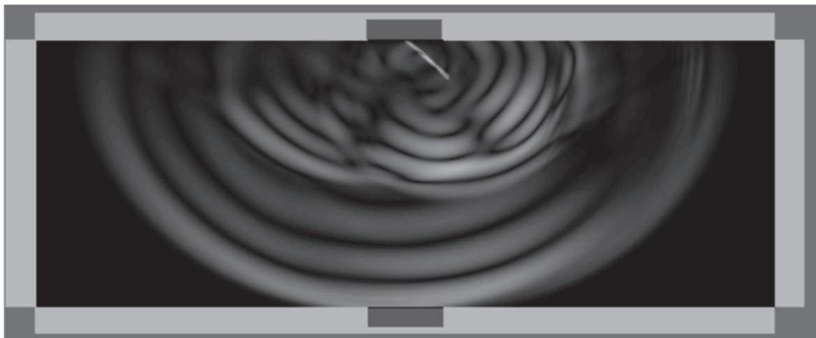
Fig. 7. Acoustic Emission Wave Propagation in fractured Material
