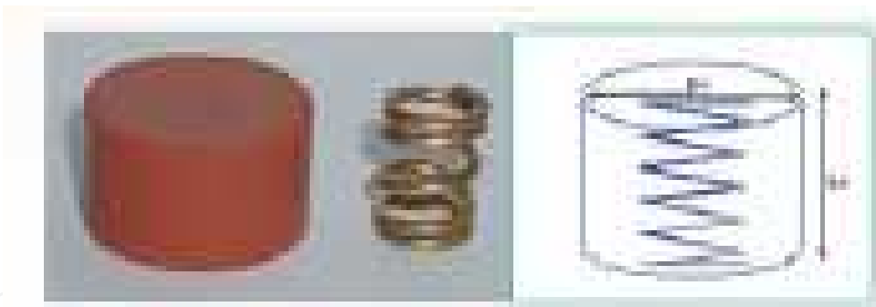
Fig. 17. Example of Composite Rubber/SMA spring damper
