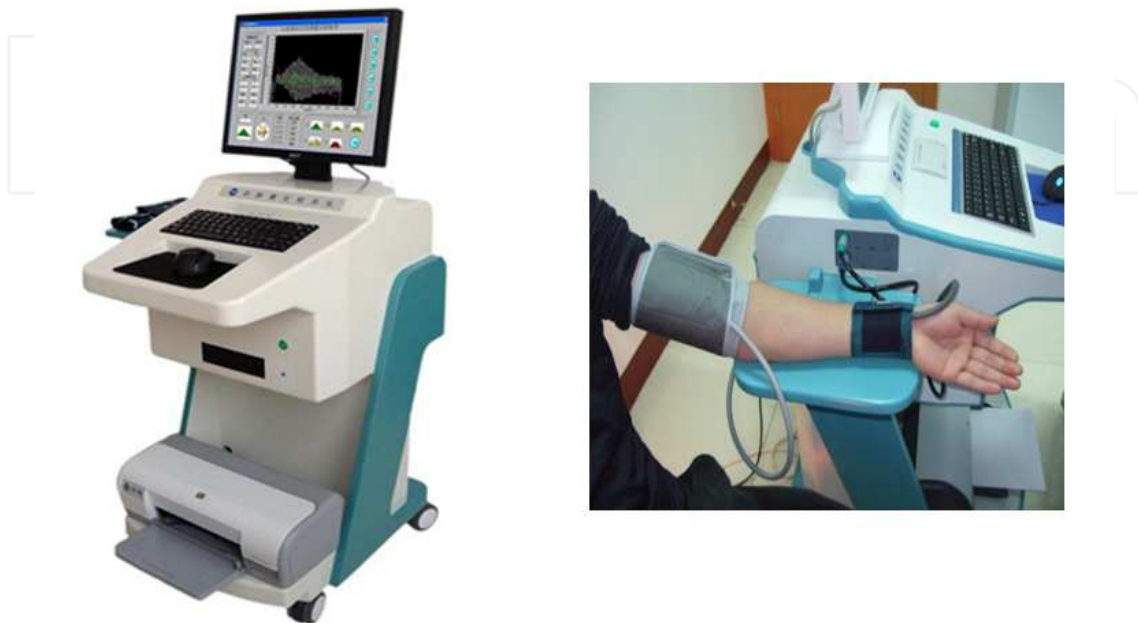
Fig. 2. The YF/XGYD artery stiffness measuring instrument and the field testing
