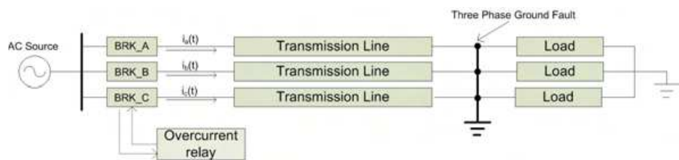
Fig. 20. One-line diagram of system with three-phase ground fault
