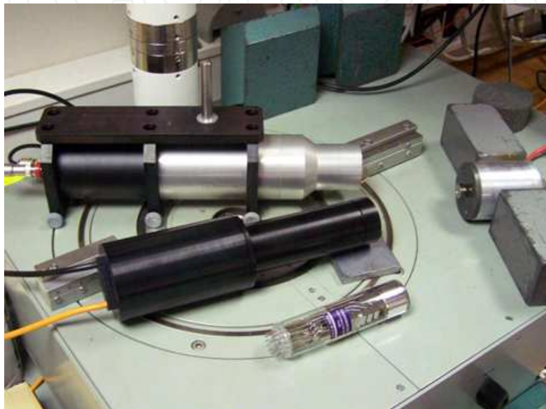
Fig. 6. High energy detector - upper, and low-energy detector - lower; and simply PMT.
