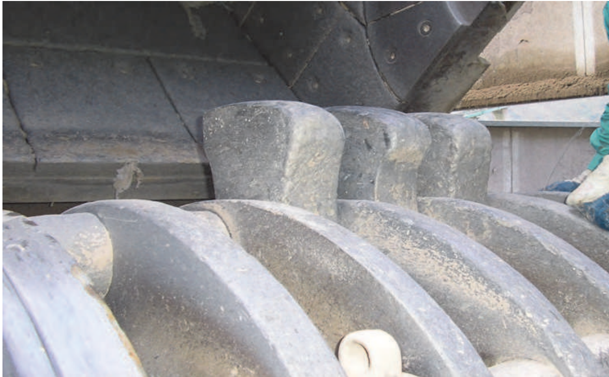
Fig. 22. Three experimental hammers in a rotary mill
