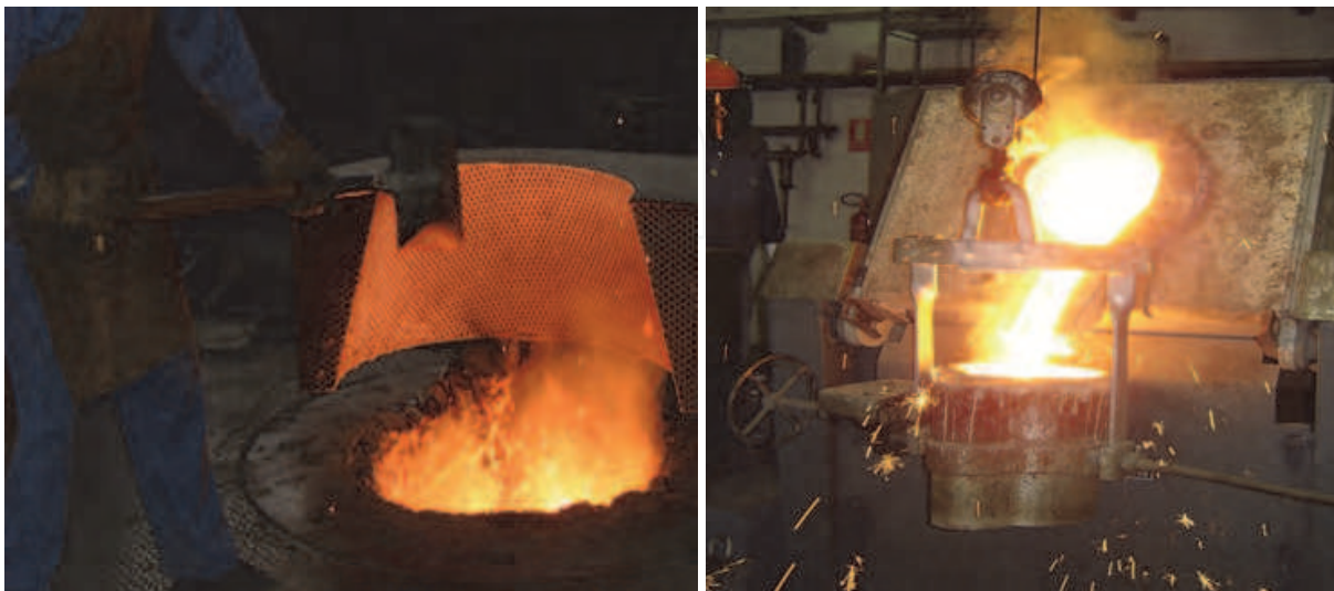
Fig. 11. Masteralloy addition and pouring of steel+carbides
