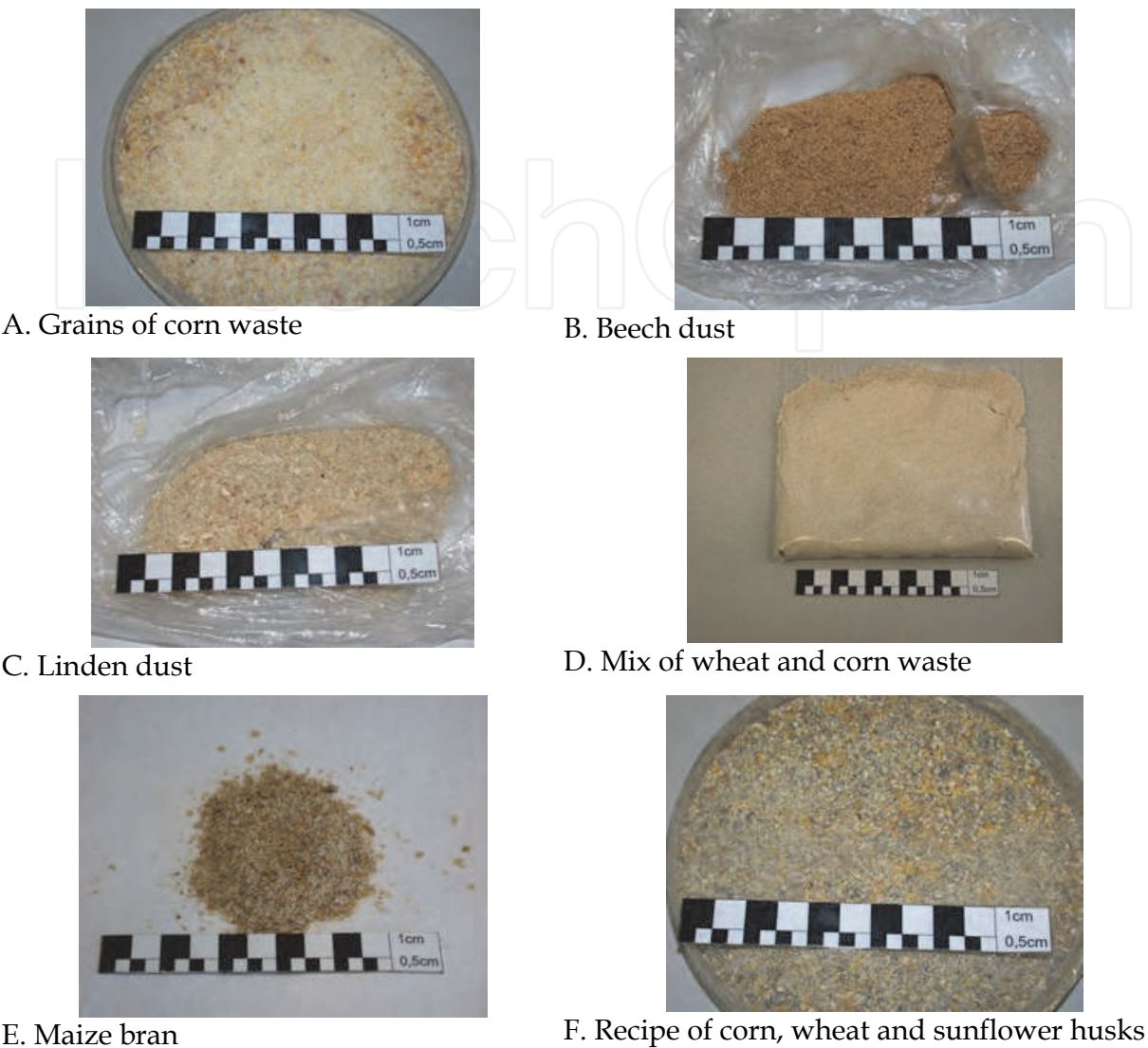
Fig. 2. Materials used in anaerobe fermentation (Cioablă, 2009)
