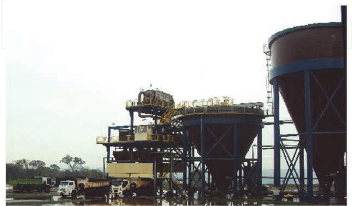
Fig. 4. System for treatment of water from gas washer to remove the ash using decanters and porous blankets.
