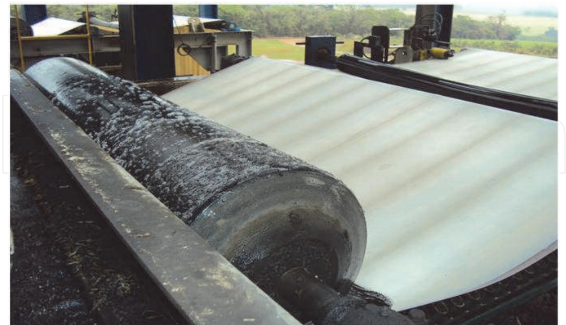
Fig. 5. Blanket type filter system (with suction strainer) to remove water and reduce moisture from the ashes
